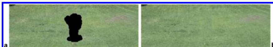
14 Background inpainting of the third video: (a) original frame; (b) inpainted background after filling in the mask
