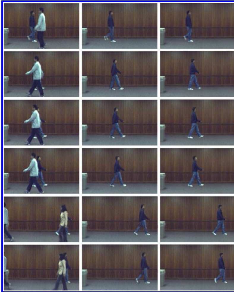
11 Comparison of the results of our algorithm with results of Venkatesh et al. 's algorithm 20 when two occluding persons, moving from right to left, are removed. The first column shows a number of original frames of the test video. The second column shows the inpainted frames using algorithm by Venkatesh et al. 20 The third column shows the results of the proposed algorithm
